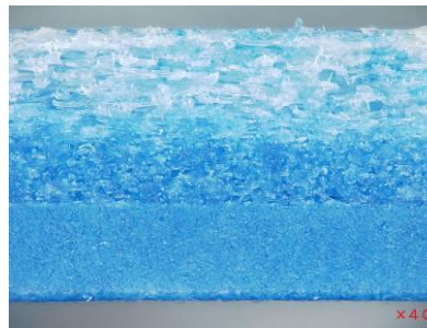
Fig3. Cross section of filter layer① (Three layers type) 【model:MF-6560】
