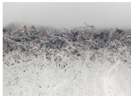
Fig2. Cross section of Eraser [Holdings of dust from erasing]
